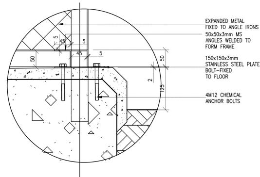
**DETAIL A: SECTION OF FIXING PLATE**
